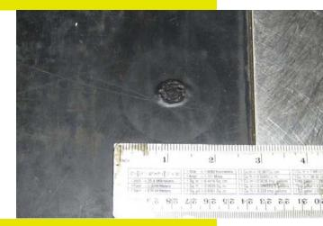
Recently a MagLite 6V 2.5 AH rechargeable Flashlight was inadvertently left switched on and standing on its lens assembly. After a short period of time a burning plastic smell was detected and traced to the flashlight. The lens area of the flashlight had become overheated and scorched the vinyl bench-top. The incident highlighted a significant fire hazard; particularly had it gone unnoticed or occurred after hours.
